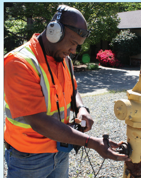
Above, Sanjay Adlam listens for a leak at a standing hydrant.
