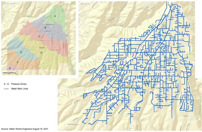
Figure 3 Paradise Irrigation District – Water Main Distribution System and Pressure Zones
